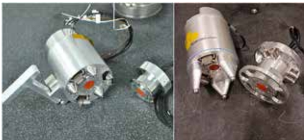
Figure 1: Manual, left, and mechanized, right, versions of the Dust Tolerant Connector.
