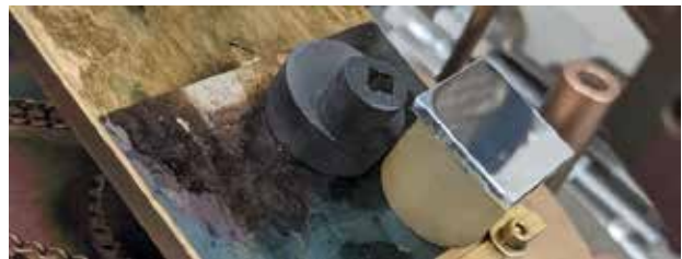
Image 1. Cold-welding test specimen before the coating is applied on the surface
