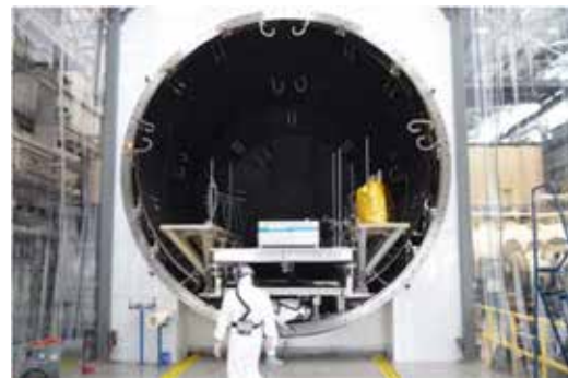
Figure 2. LSS Chamber with Regolith Bed Visible
