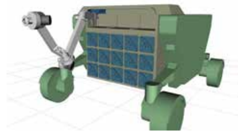
Figure 2: Astrolab’s 6-DoF Robotic Arm and Payload Mezzanine attached to the FLEX rover.
