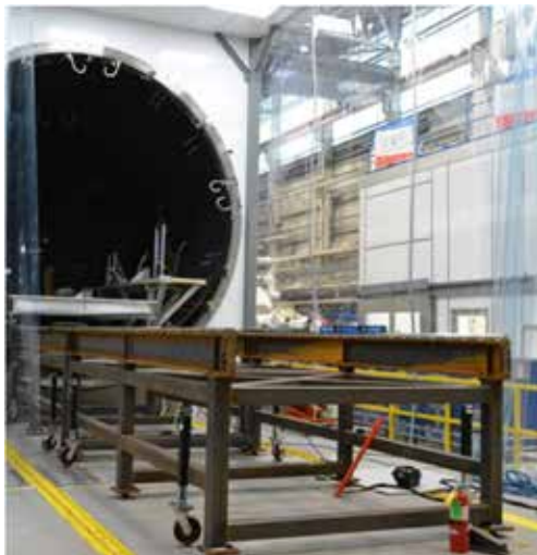
Figure 1. LSS Chamber and External Rail System
