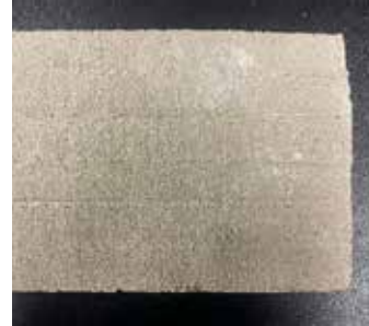
Figure 1. 3D printed sulfur concrete specimen at LSU
