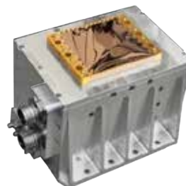
Figure 2: Fully integrated Nightingale I payload supporting LunaNet communications
