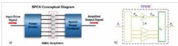
Figure 1. a) Spatial Power Combining Amplifier Diagram (SPCA). b) MMIC on-chip power combining diagram. P_i : input power, P_o : output power, L_o : output load.
