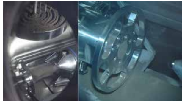
Figure 2: DTC vacuum testing in the presence of JSC-1AF lunar simulant. Left, DTC and the regolith dispenser before the test. Right, dust covered female side of the connector during testing.
